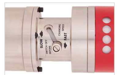
FIGURE 10 – 'FAST' speed above, 'SLOW' speed below.
