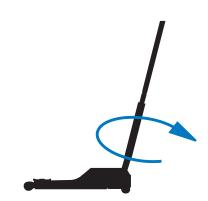
Clockwise turn the handle to completely close the release valve.
