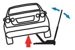
Pumping the handle up and down to lift the vehicle.
