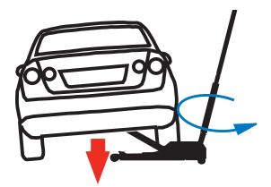
Counter-clockwise and slowly rotate the handle to lower the vehicle.
