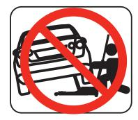
This hydraulic trolley jack should be used for lifting and lowering only; The raised vehicle should be supported on two vehicle support stands.
