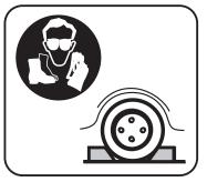
Personal protection equipment is required before operation. The unlifted wheels of the vehicle should be chocked.
