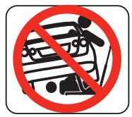
No person should remain in a vehicle that is being lifted. No person should get bodily under a vehicle that is supported by a hydraulic trolley jack.
