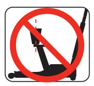
The load should be centrally located on the head cap.
