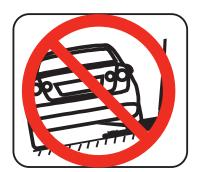
The trolley jack should be used on a hard level surface and be free to roll during lifting and lowering.
