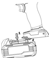
1. Always switch off the machine before insertion or removal of the battery pack.
