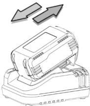
4. Push the battery pack into place and make sure the red light on the charger is "ON". The battery pack is now starting the charging cycle.
